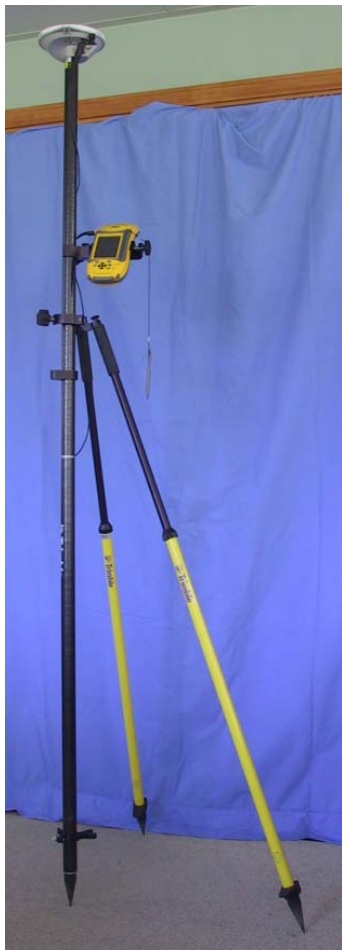
Zephyr mounted on 2-part range pole, which is 2.0 m from the base of the antenna to the point at the bottom.
