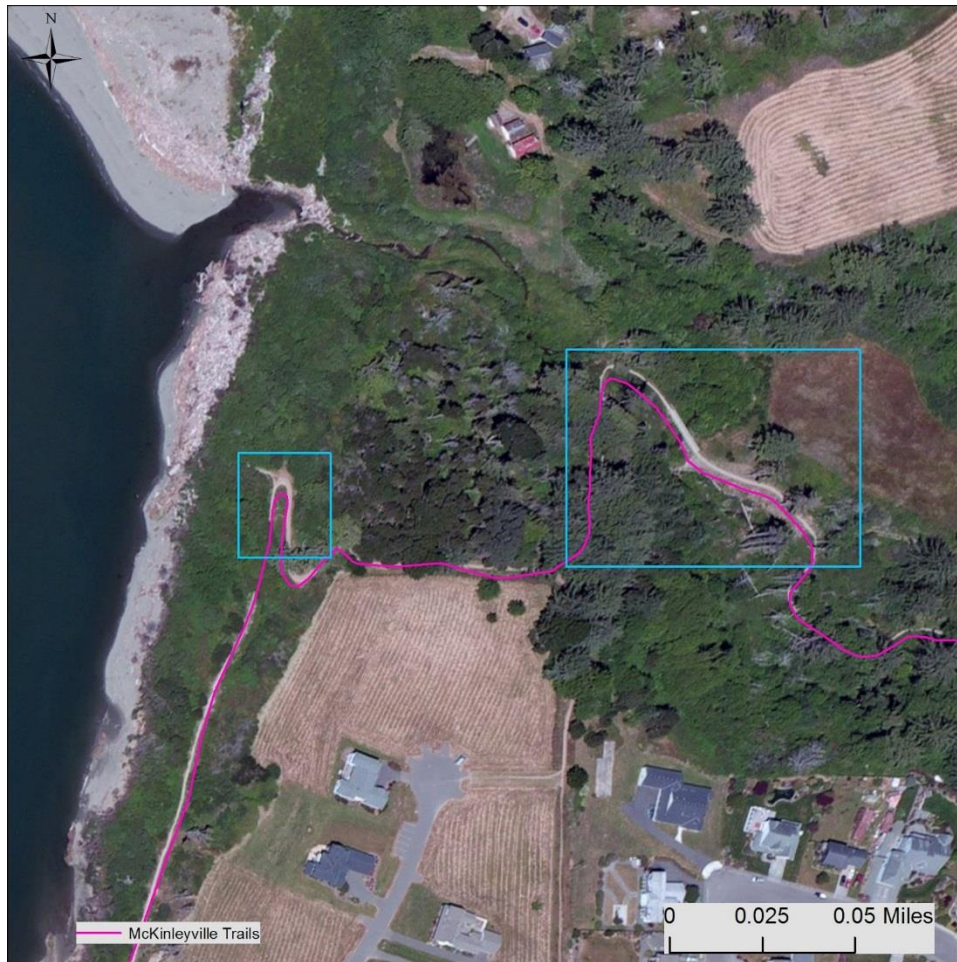
Figure 4. The blue squares highlight areas where the trail layer is different from the basemap. Because of the data collection method used, this amount of error is to be expected.
